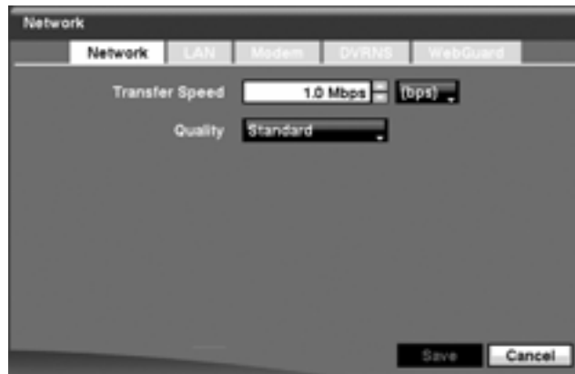
Figure 3-24 Network Setup Screen
